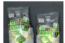
HALCON's local deformable matching finds objects with surface deformations.
