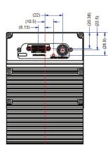
NOTES: 1. UNITS: MILLIMETERS. 2. IMAGE AREA IS ALIGNED TO DATUMS A B & C.
