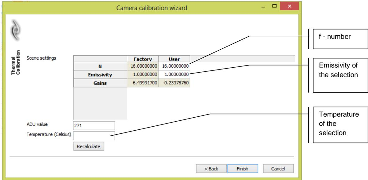
Figure 5-40 Thermal calibration (InGaAs)
