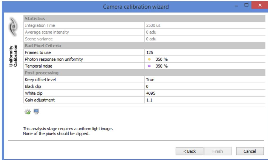
Figure 5-32 Two point calibration – Bad pixel criteria and post processing
