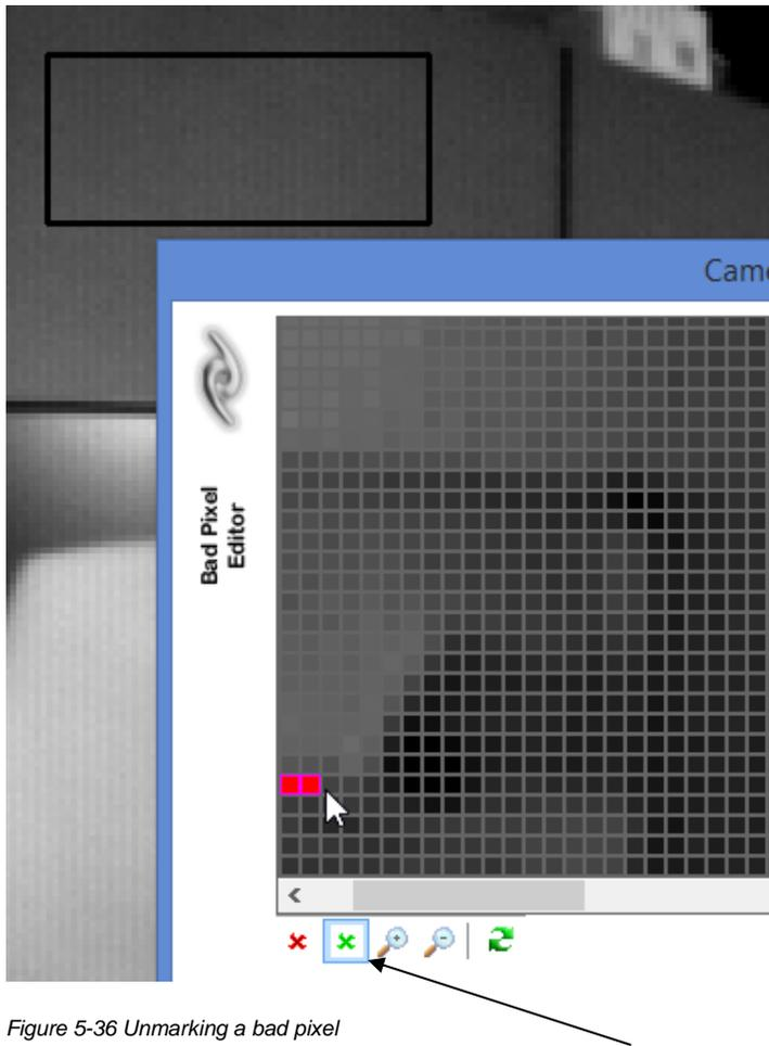
Figure 5-36 Unmarking a bad pixel
