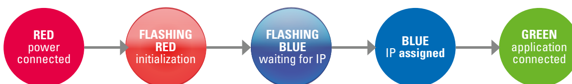
Device status indicated by external LED
