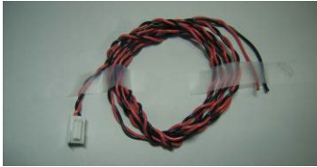
(1) 5V DC power supply cable (For CIS Sensor drive)
