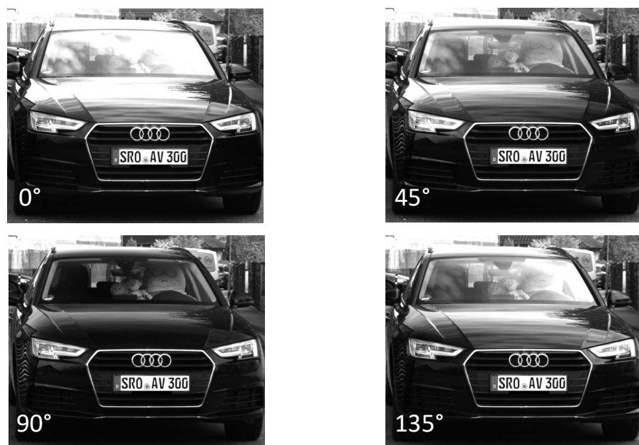
Figure 3: Polarization angle versus image brightness in sub-images
