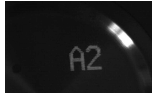
395nm UV Light with MidOpt BP470 Blue Bandpass Filter
