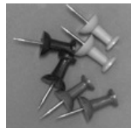
Blue Bandpass Filter highlights blue push pin
