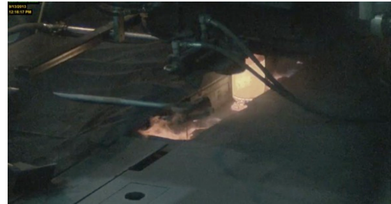
Reduce intensity, saturation & interfering red channels with a neutral density filter in combination with a shortpass filter
