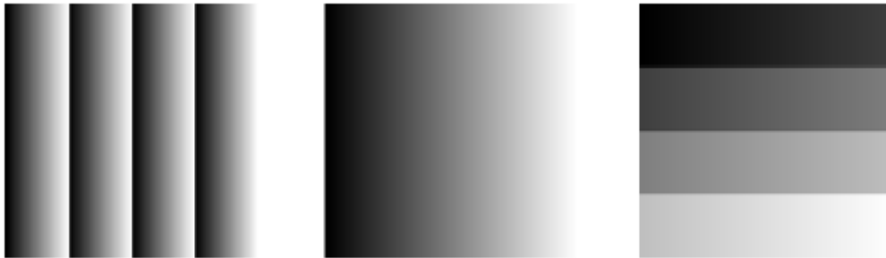
Figure 31: Ramp test images: 8 bit output (left), 10 bit output (middle), 12 (right)
