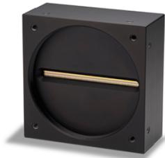
Based on Teledyne e2v's trilinear color CMOS sensor, the new Piranha4 8k camera provides outstanding signal-to-noise for color imaging. The camera has 8k resolution with a  $7.5 \mu\text{m} \times 7.5 \mu\text{m}$  pixel size for optimized optical design, delivering a maximum line rate of 33 kHz x 3, and a Camera Link interface.
