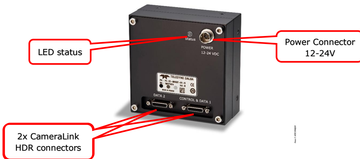
Figure 21: Camera I / O Connectors
