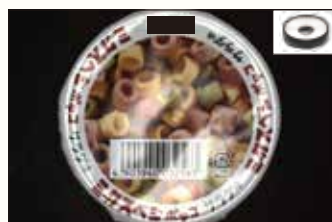
With Ring Lights, reflection from the packaging film makes it difficult to perform stable examination.
