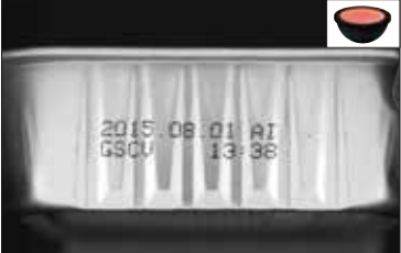
Imaging with Dome Light captures reflections from the bumps on the container.
