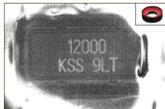
With Ring Lights, reflection from the embossed tape surface makes it difficult to perform stable examination.
