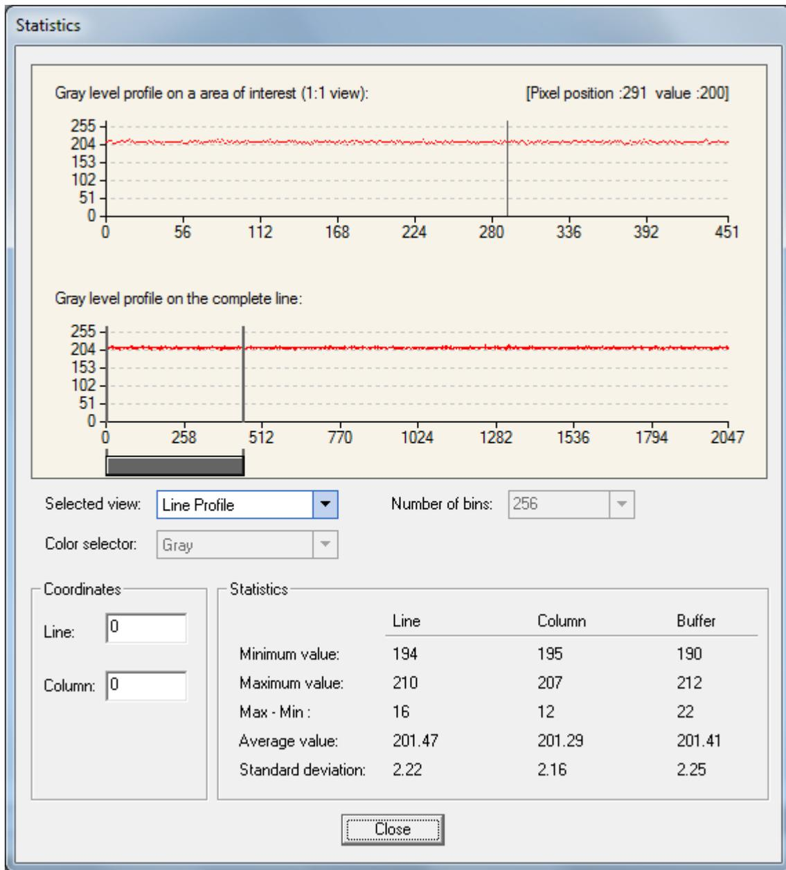
Figure 4 A line profile of a white uniform target after PRNU is calibrated.
