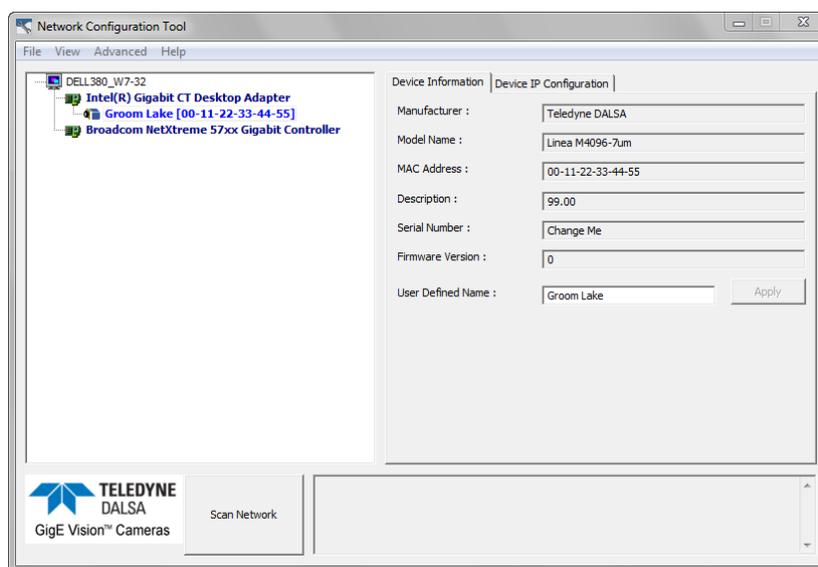
Run the tool from the Windows Start menu: **Start•Programs•Teledyne DALSA•Sapera Network Imaging Package•Dalsa Network Configuration Tool**. Verify the camera appears as a child of the NIC card it is connected to. By default the camera is identified by its serial number if no user defined name has been assigned.
