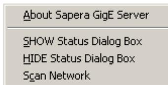
Click on Show Status to open a window listing all devices connected to the host system. Each GigE device is listed by name along with important information such as the assigned IP address and device MAC address. The screen shot below shows a connected Linea GigE with no networking problems.
