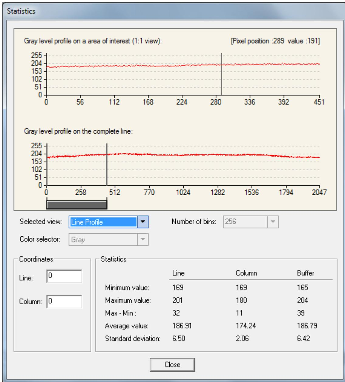
Figure 1 A line profile of a bare image of a white and uniform object.
