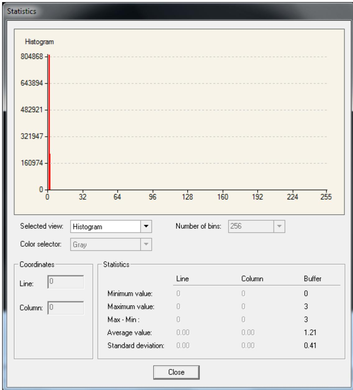
Figure 3 A histogram of a dark image after FPN has calibrated.
