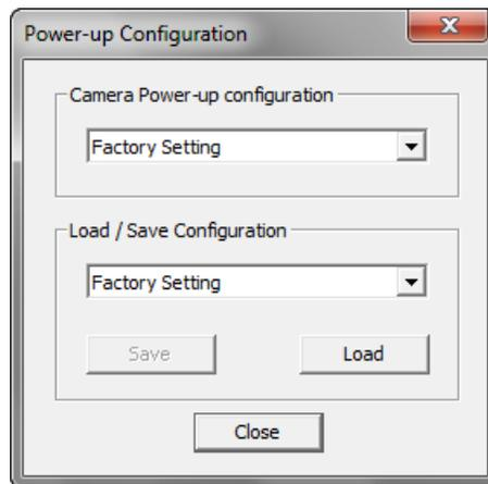
CamExpert provides a dialog box which combines the features to select the camera power up state and for the user to save or load a camera state from Linea GigE memory.
